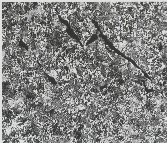
Fig. 3: The microstructure of the bolt consists largely of pearlite, with some ferrite, and slag inclusions elongated by forging. This is a steel of around 0.6% carbon. Elements of armour from this garniture were made from similar steel. Magnification: x 135.
