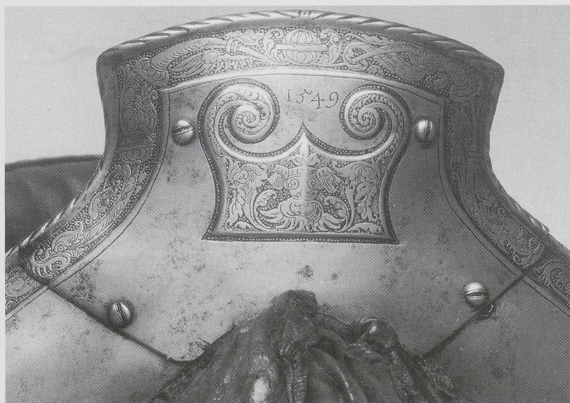
Fig. 1: Front view of a saddle dated 1549 in the Wallace Collection, London, cat. no. A409. The four threaded bolts which fasten the saddle-steels to the saddle are clearly visible. The lower one on the right of the picture was examined metallographically in cross-section of its inside end (Reproduced by permission of the Trustees of the Wallace Collection).
